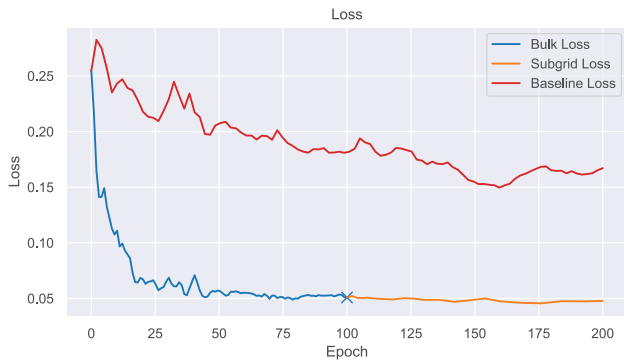
Figure 7: Loss plot for the plume example at resolution 1024^2 . We visualize the density mean squared error, instead of the full energy function \Phi . While the baseline fails to optimize after 200 epochs, our method decreases the loss significantly. For our method, the first 100 epochs correspond to the down-sampled bulk optimization. Later 100 epochs correspond to the subgrid optimization.
